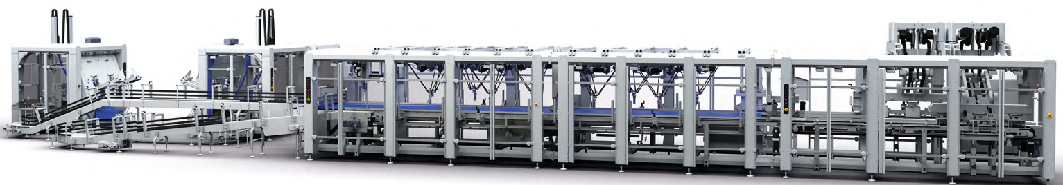
Monobloc robotized loading and closing unit (Source: Cama Group)
