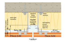
Total thickness of the Piterak® SLIM cladding system: - without insulation: 95 mm;
