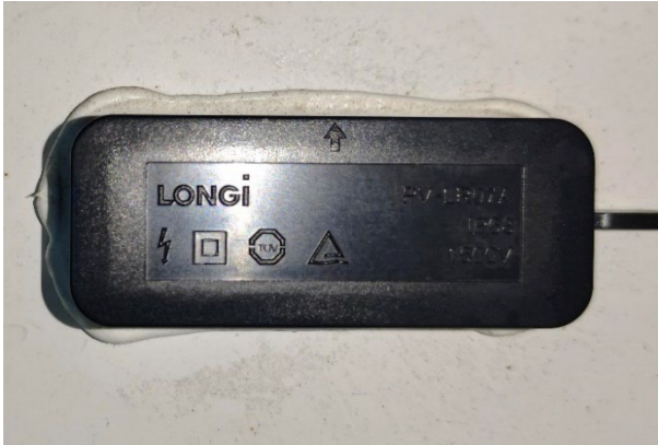
Junction box (PV-LR07A)
