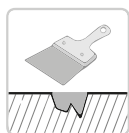
Stuccare i buchi/ Fill the holes
