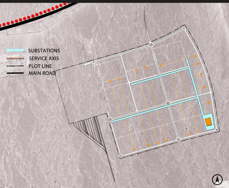
The main technical services will be located along the service corridor. Services included: - stp/etp - power substations -gas supply - solid waste collection - water storage
