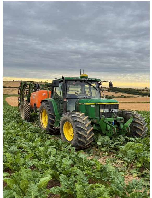
John Deere 6410 working in sugar beet with an Amazone UG 3000 Super sprayer equipped with a 21-metre boom
