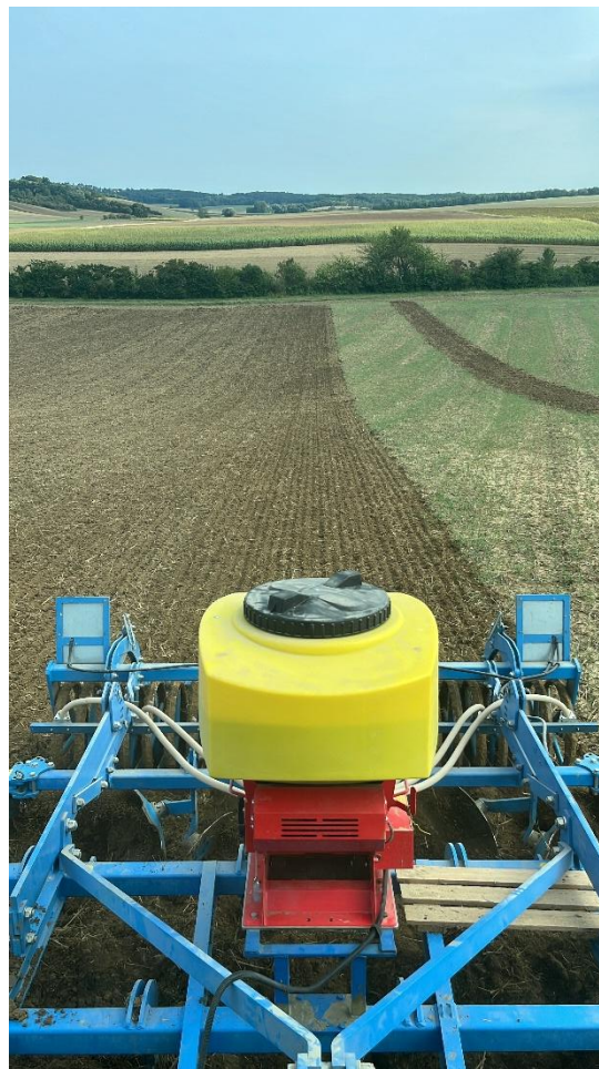
Cover crop sowing in autumn. Simon uses a pneumatic seeder mounted on the Lemken Rubin disc harrow
