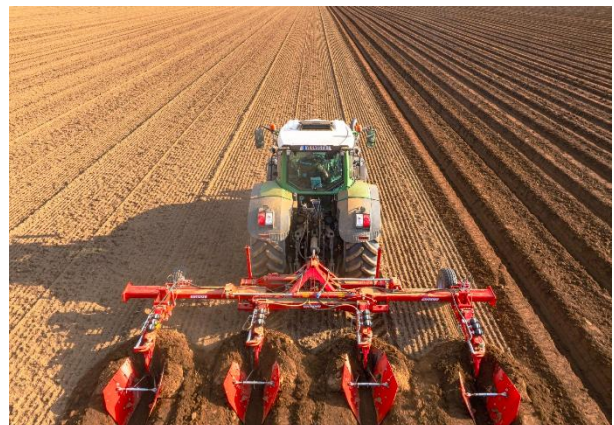
Preparation of the potato seedbed using a Grimme BFL combined with the Fendt 939. The ridges are formed using bodyies with long side mouldboards, which help keep the soil loose along the sides and prevent it from falling back into the newly formed furrow
