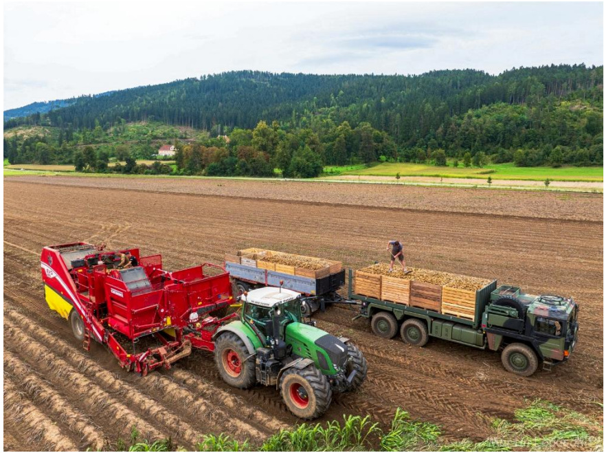
Potato harvesting with a Grimme EVO coupled to a Fendt 939. At least one person is required beside the sorting belt to monitor the process closely and remove any unwanted material from the crop
