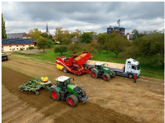
Fendt 1050 with an Amazone Centaur trailed cultivator, working immediately after the potato harvest. In the background, a Fendt 939 and a Grimme EVO trailed potato harvester unload the crop into bins placed on the truck trailer
